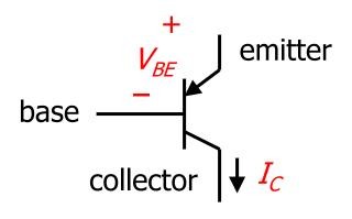
$$\Rightarrow V_{BE} = \frac{kT}{q} \ln \frac{I_C}{I_S} \qquad I_S = A_E C T^{\eta} \exp \left(-\frac{qV_{g0}}{kT}\right)$$
